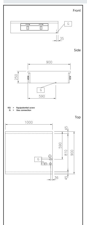
Gas Gas Power: 40 kW Gas Type Option: Gas Inlet: 1/2" **Key Information:** External dimensions, Width: 1000 mm 900 mm External dimensions, Depth: External dimensions, Height: 250 mm Net weight: 82 kg Configuration: Two-Side Operated;Top ISO 9001; ISO 14001 - ISO 9001; ISO 14001 kW Front Burners Power: **Back Burners Power:** 10 - 10 kW **Back Burners Dimension -**Ø 70 Ø 70 Front Burners Dimension -
